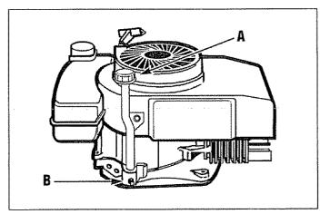
Figure 27: Dipstick (A) and oil drain plug (B).
